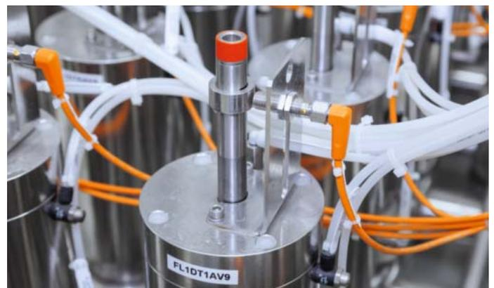
Position feedback: The IFT203 inductive sensor monitors the valve stem and signals to the controller if the valve is open.
