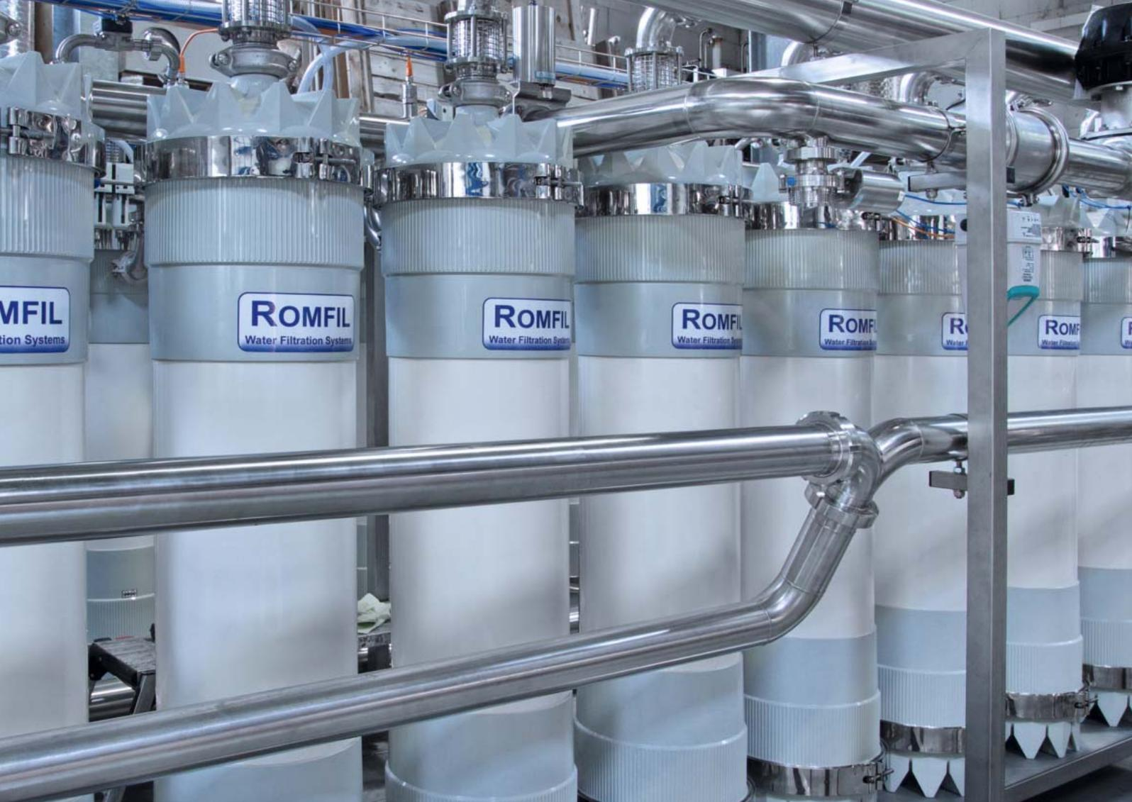
*The crossflow filter system filters up to 300 cubic metres of water per hour.*
