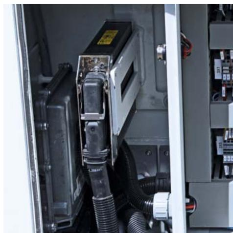
The powerful type CR7 SafetyController from the ecomatmobile series from ifm electronic built into the vehicle ensures safety in mobile applications.
