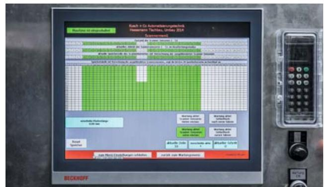
*The controller receives an image of the workpiece from the sensors and controls the lowering of the individual sanding segments.*
