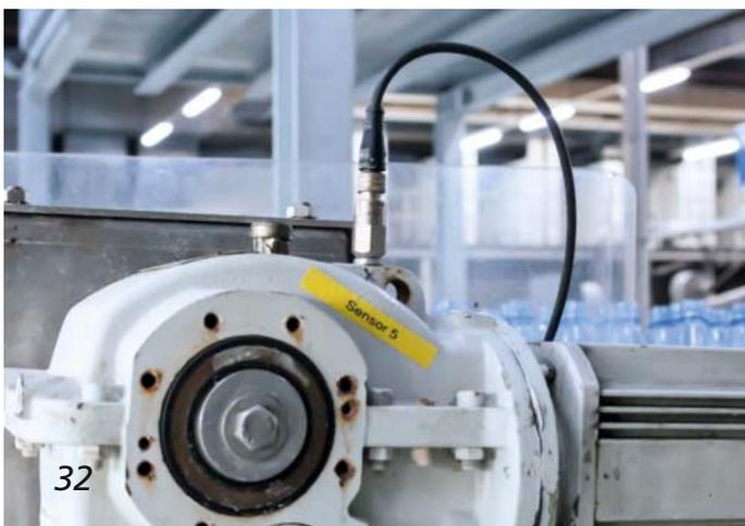
The pre-alarm and main alarm are provided via switching outputs and, as is the case at Hassia, via light indicators. The evaluation unit communicates for example with the machine controller or the process control level via Ethernet TCP/IP.
