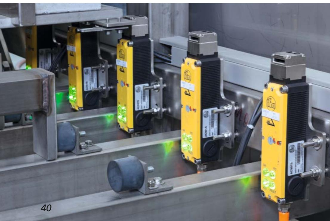
*Thanks to these safety-related AS-i door switches with guard locking the pull-outs cannot be opened unintentionally while cleaning is in process.*
