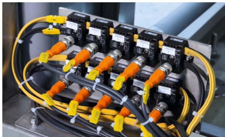
*Passive flat cable insulation displacement connectors for the connection of intelligent AS-i sensors / actuators to the yellow flat cable.*
