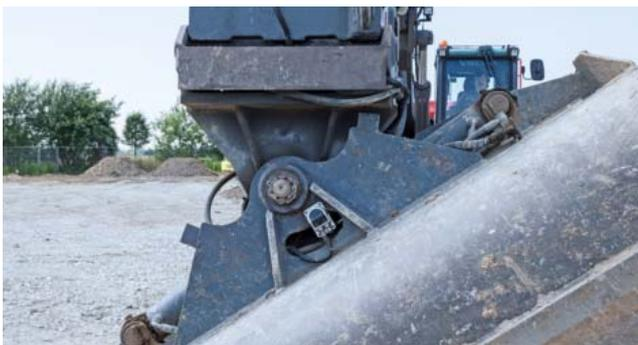
The lateral inclination of the excavator bucket is also taken into consideration for the calculation.
