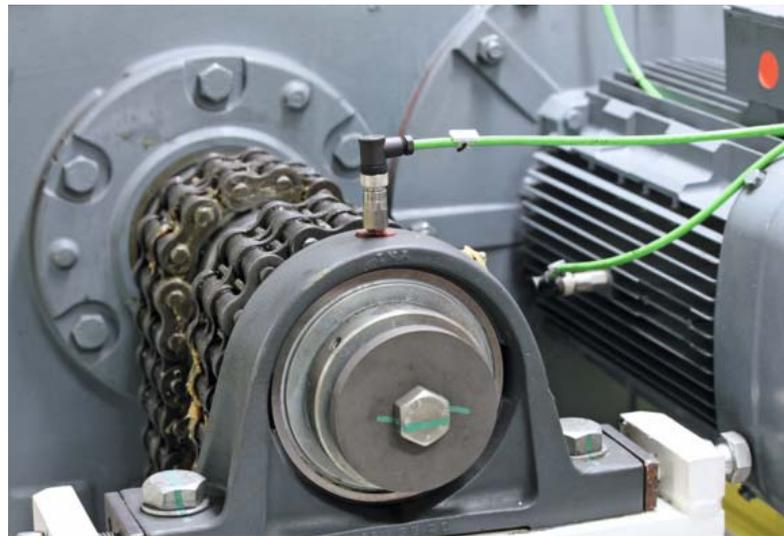
*Vibration sensors monitor bearing and gear. Wear and tear is detected in time.*
