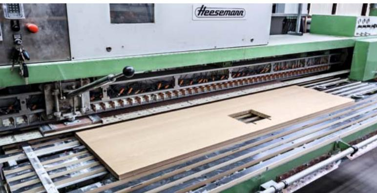
*53 lowerable pressure shoe segments adapt to the surface of the workpiece geometry during sanding. That avoids undesired rounded sanding edges.*
