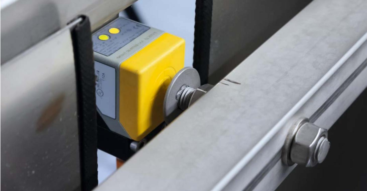
*"Safety at Work": This fail-safe inductive sensor for position monitoring is connected to the controller via AS-i.*
