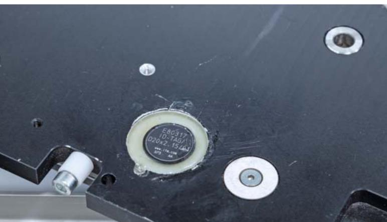
The ID tag chip is installed at the bottom of the workpiece carrier. The chip can store up to 224 bits.
